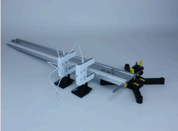
Fasten photogates to adapter plate using spacer bolts
